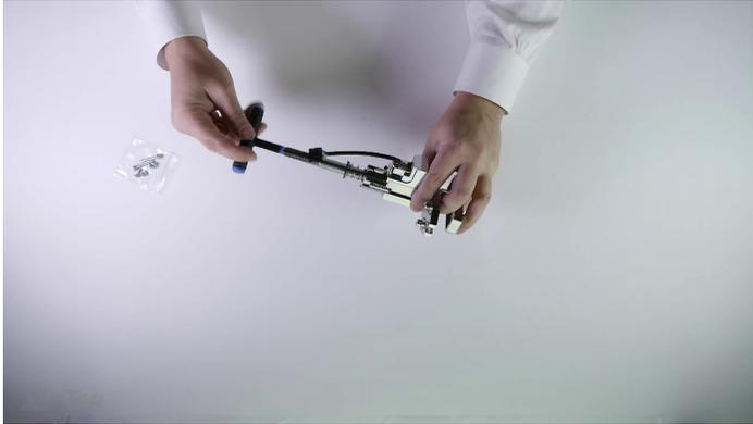
**6. Connect the latch module connector to the latch module wire harness, then the latch module wire harness to the CPU.**
