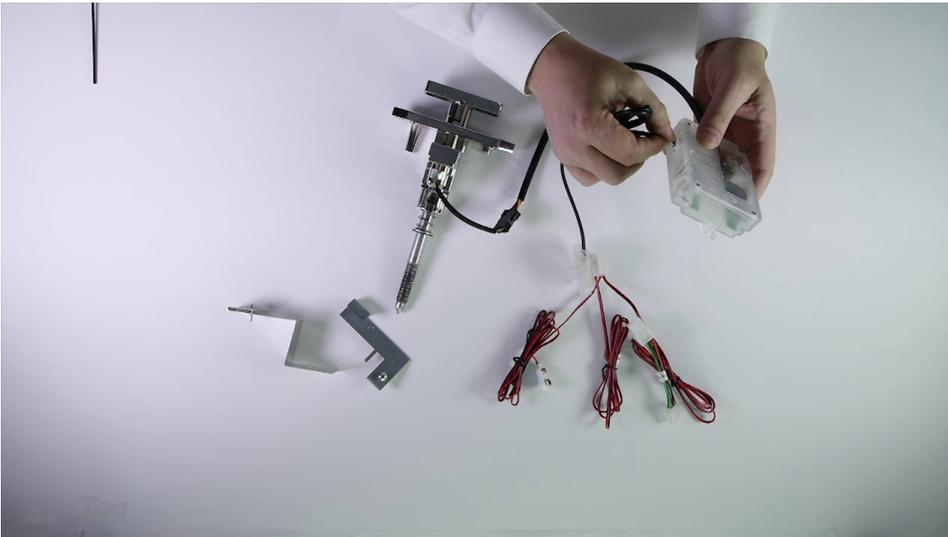
**9. Connect the power wire harness 6-pin connector to the CPU.**
