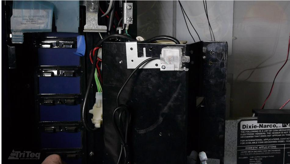
Use the enclosed self-tapping screw to attach the bracket to the frame. A cordless screwdriver may help in this application.
