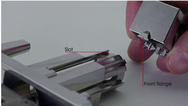
Line up the rear flange with the slot on the housing and complete sliding the latch module into the housing while both the front and rear flanges are in the housing slot.
