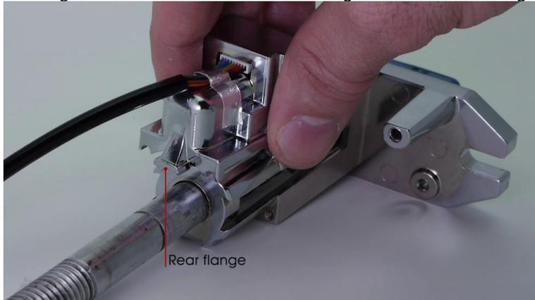
The latch module will be fully seated in the housing only when both the front flange is fully seated in the notch at the end of the slot, and the latch modules legs are fully seated at the rear of the housing at the fastening location.
