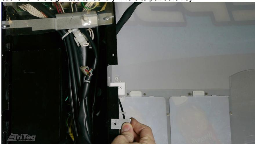
In a final example, the receiver is mounted inside the product delivery chute. The key will be pointed into the product delivery chute to operate the lock.
