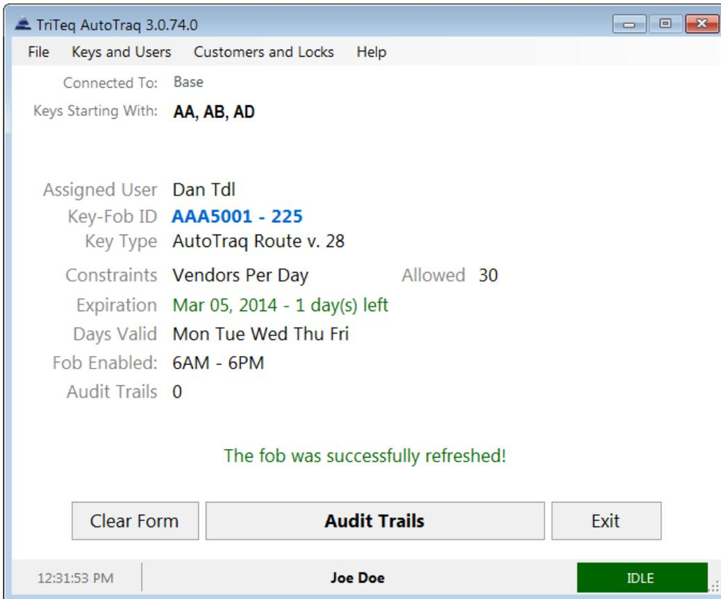
To refresh an AutoTraq fob, place the fob in the cradle and press on the button.
