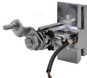
**5. Attach the latch module to the SnackIQ housing.** Slide the latch module on the housing by lining up the front flange on the latch module with the slot on the housing and begin to slowly slide the flange of the module into the housing slot.
